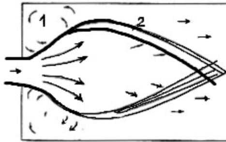
Fig. 1. Rapid flow spreading in wide channels: 1—whirlpool, 2—oblique hydraulics jumps
